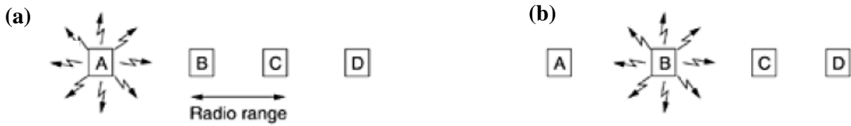
Figure 2.1. (a) Hidden node problem (b) exposed node problem.
